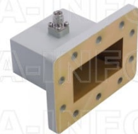
229WCASM Right Angle Rectangular Waveguide to Coaxial Adapter 3.3-4.9GHz WR229 to SMA Male
